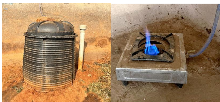
Image 2: Bio-gas Unit at beneficiary HH
